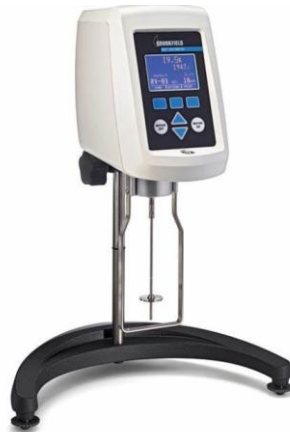
Figure 15 Image of a Brookfield viscometer for measuring viscosity
