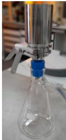
Figure 9 Kitasato flask for 1 \mu\text{m} filtration of the liquid effluent
