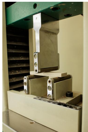
Figure 7 Image of the testing device for performing three-point bending
