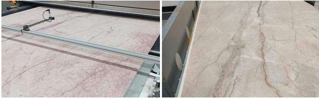
Figure 8 Image of an industrial tile after the decoration process (left) and a fired industrial tile (right)
