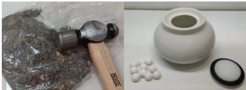
Figure 3 Image of manual grinding (left) and alumina jar and grinding balls (right)
